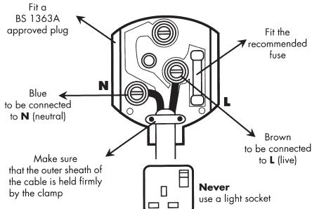
As the colours of the wires in the mains lead of this appliance may not correspond with the coloured markings identifying the terminals in your plug, proceed as follows:
